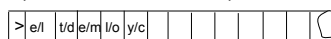
Figure 1.5: To simulate a machine M with alphabet \Gamma that has tapes infinite in both directions, we use a machine \tilde{M} with alphabet \Gamma^2 whose tapes encode the “folded” version of M 's tapes.
